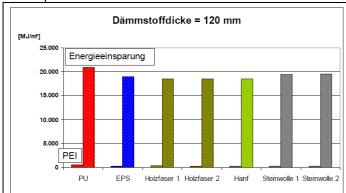
Energieeinsparung (energy savings), PEI (primary energy content), PU (Polyurethane), Holzfaser (wood fibre), Hanf (hemp), Steinwolle (stone wool)
