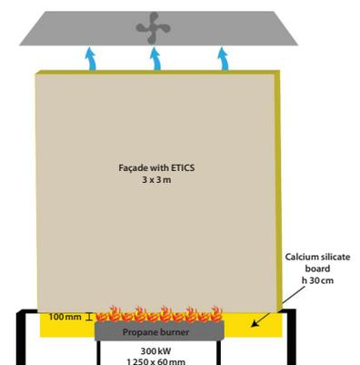
Experimental test method: equipment and test conditions
